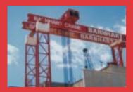
Barnhart's newest addition to their heavy rigging arsenal had its coming out party in the heart of Virginia this summer. The 500 Ton Hoist debuted atop the Modular Lift Tower (MLT) in Fluvanna County. In the past, the Modular Lift Tower has employed one or more 450 ton capacity strand jacks as the hoisting mechanism. The strand jacks are reliable, but slow and are not ideal for duty cycle work. Enter the new 500 Ton Hoist.
