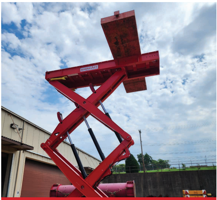
Each lifting table can lift a 50,000-pound load from just 40 inches above the ground and push it up to a final height of 26 feet in a continuous movement.
