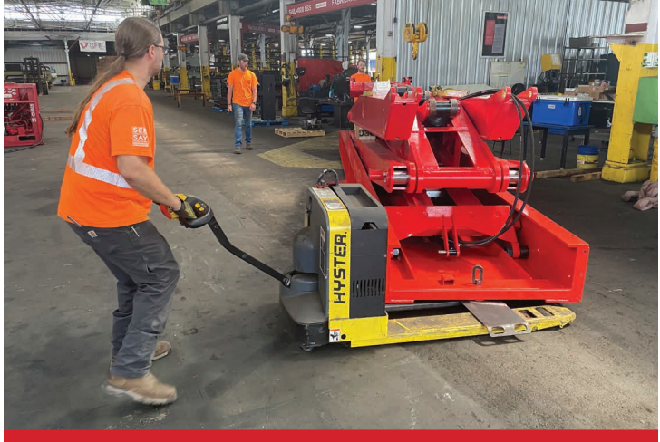
Barnhart can engineer and fabricate new tools to meet customer demands. Above, the lifting table is moved from the fabrication shop for further testing.
