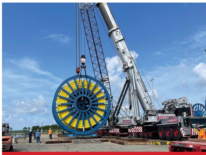
The Mobile team tackles a 300-ton and 600-ton crane lift of an ocean floor umbilical reel at Mobile Middle Bay Port.
