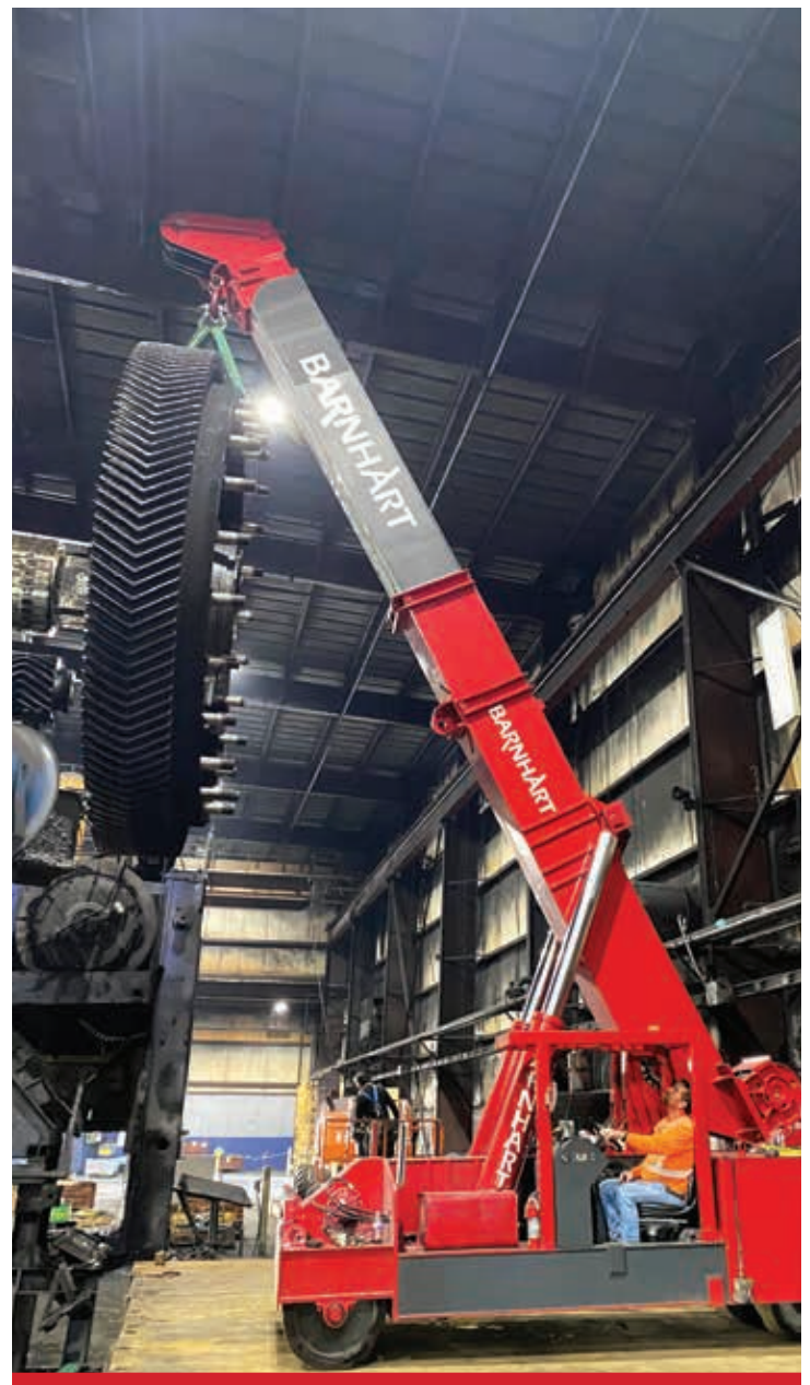
An operator uses a Mobilift to remove and replace an 80,000-pound flywheel for a press at a forge/heavy manufacturing facility.
