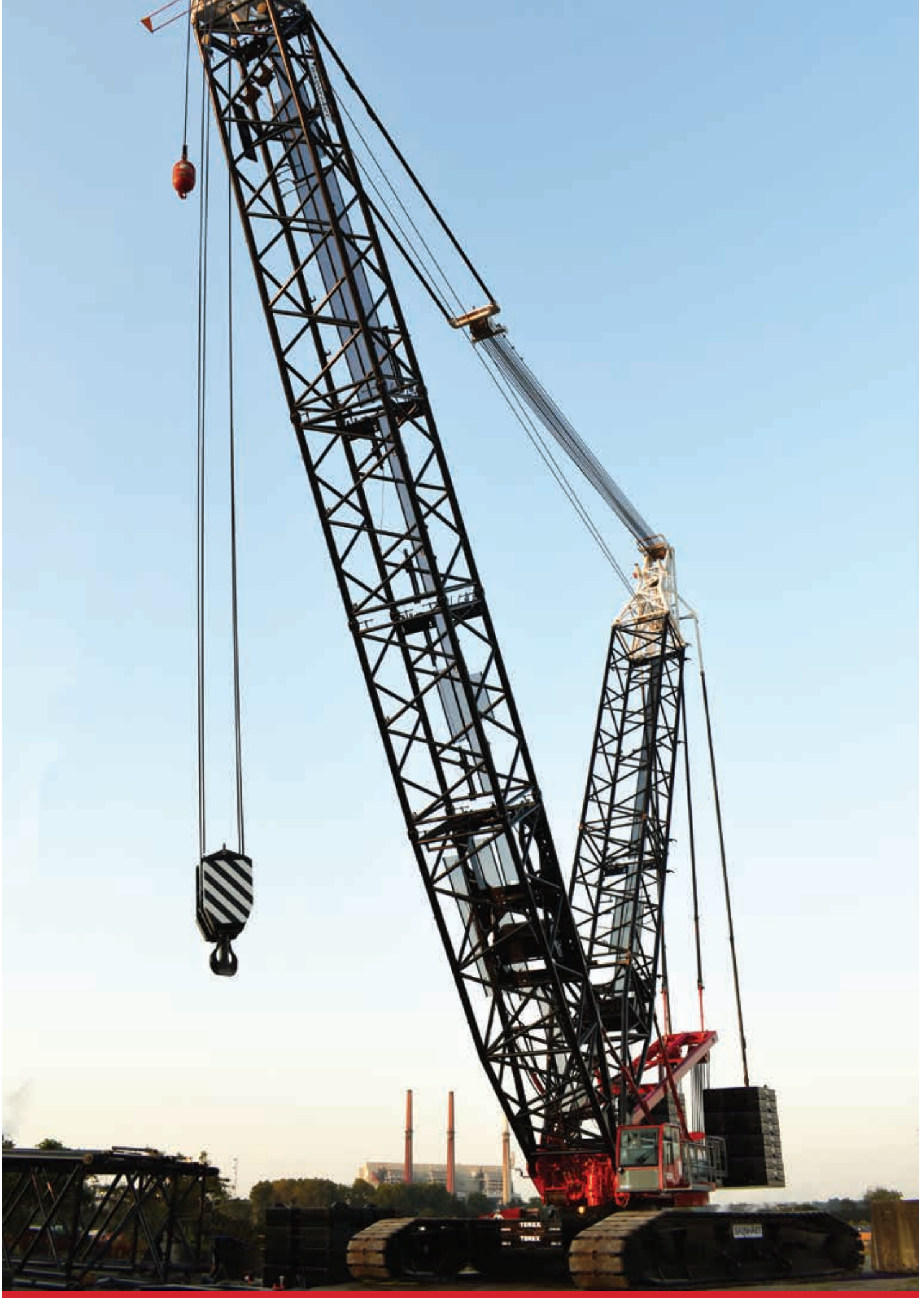
A DeMag CC2800-1 is parked at Barnhart's President's Island facility for assembly and testing before deployment to a project.
