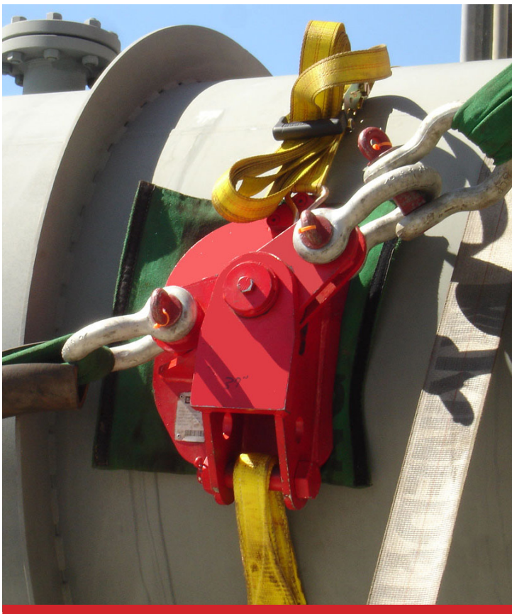
Trunnions can be adjusted to meet a variety of situations and diameters.
