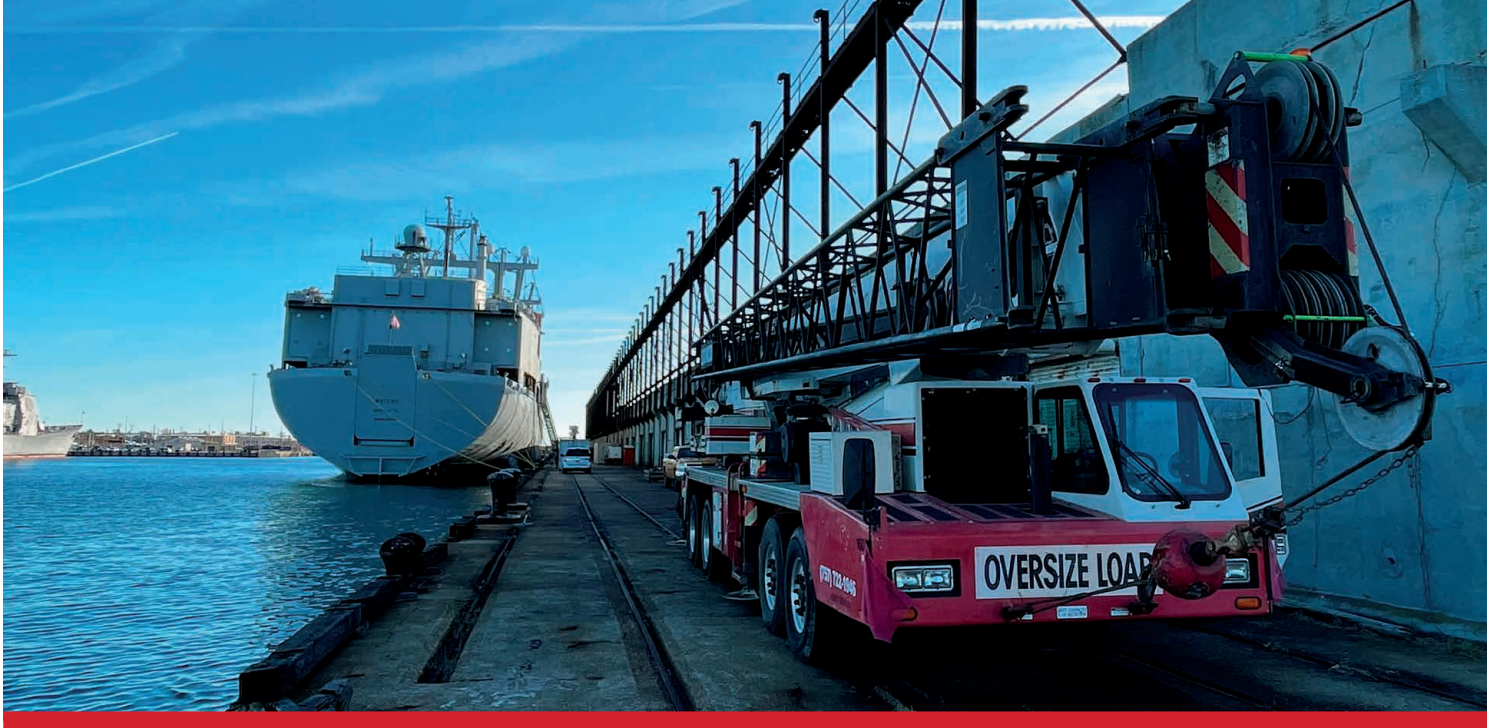
An all-terrain crane mobilized to Naval Station Norfolk to load supplies to the USS Wright.
