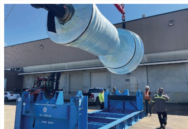
The Memphis crew loads the rotor onto a shipping stand.
