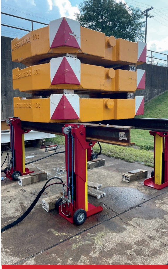
Barnhart's 15 Kip Jack Master, with a minimal toe height of 5", lifts heavy loads effortlessly, even in tight spaces.
